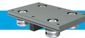
HepcoMotion Standard SL2 Carriages are available to suit all sizes of stainless steel [Double Edge Slides](#). Carriage Plates are precision machined from aluminium alloy and are supplied with a proprietary U.S. Dept. of Agriculture approved coating providing corrosion resistance better than many stainless steels. Fully stainless steel carriages are available to special order according to materials available.
